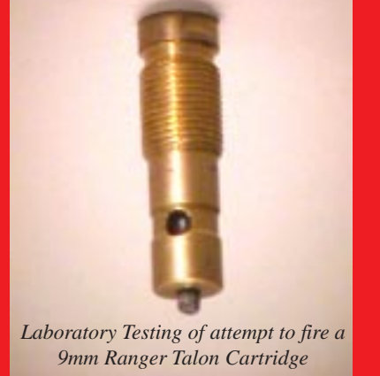
Note projectile stuck at bottom of Conversion Device - DANGER - DO NOT ATTEMPT TO REPLICATE
